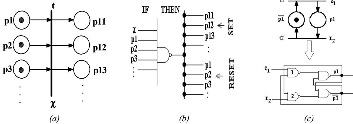
Fig. 3. a). A transition in SAPN. b). Implementation of the transition, b). Implementation of transitions  $t_1$  and  $t_2$  of Fig. 2.(c).
