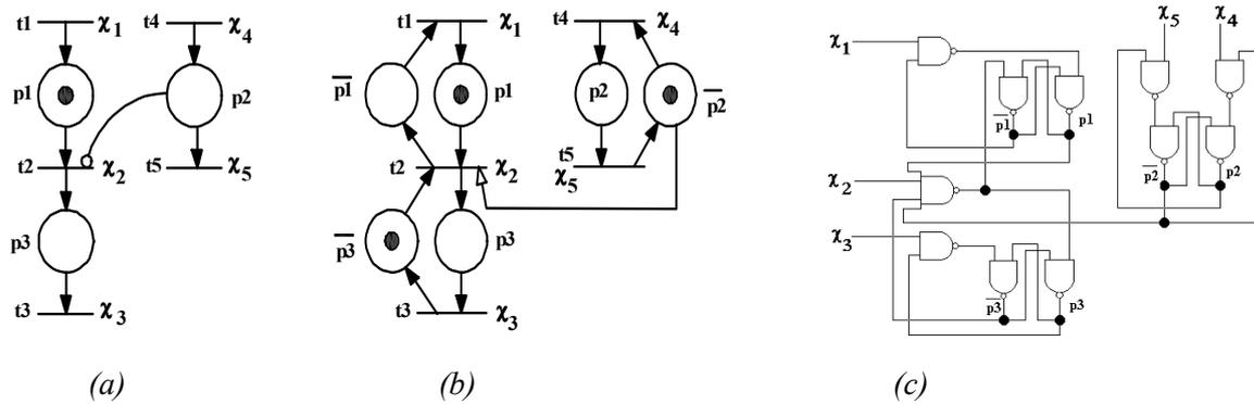
Fig. 6. a). An inhibitor arc,  $In(p_2, t_2)$ , in an SAPN. b). The complement places of places  $p_1$ ,  $p_2$  and  $p_3$ . c). Hardware implementation of the SAPN shown in Fig. 6.(b).
