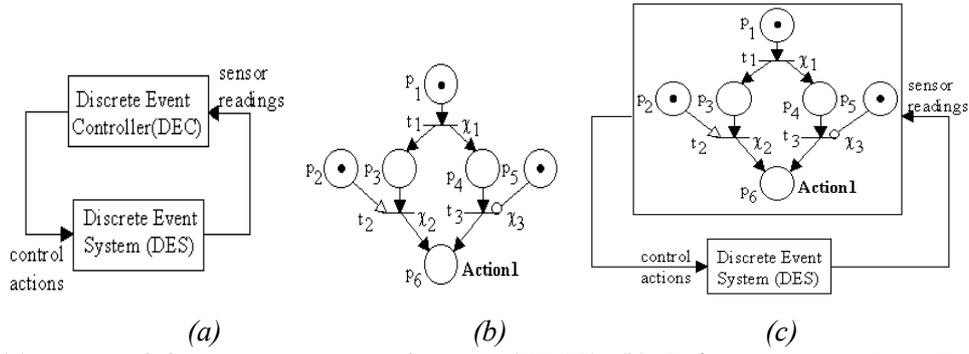
Fig. 1. (a). A typical discrete event control system (DECS). (b). Safe Automation Petri Net (SAPN). (c). APN used as a controller in a DECS.
