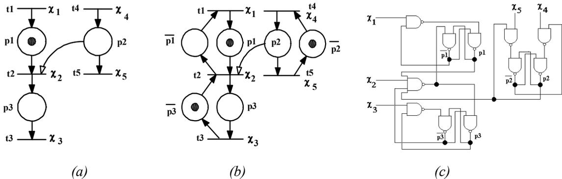
Fig. 5. a). An enabling arc,  $En(p_2, t_2)$ , in an SAPN. b). The complement places of places  $p_1$ ,  $p_2$  and  $p_3$ . c). Hardware implementation of the SAPN shown in Fig. 5.(b).
