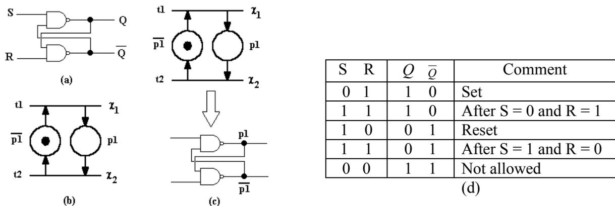
Fig. 2. a). An SR-flip-flop, b) an SAPN, c) the implementation of places. d). The truth table of the SR-flip-flop,
