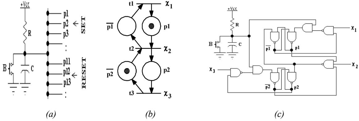
Fig. 4. a). Setting-up the initial marking. b). An example SAPN. c). Setting-up the initial marking of the SAPN shown in Fig. 4.(b).
